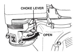
Figure 21. Choke Lever (Open Position)
